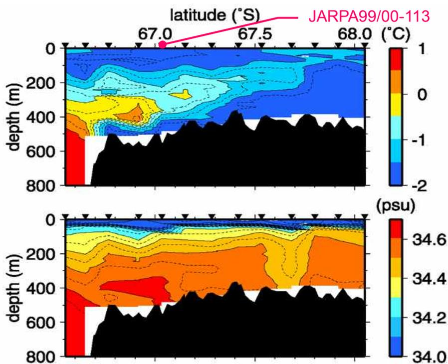
Fig. 10. XCTD sections in the Prydz Bay.
