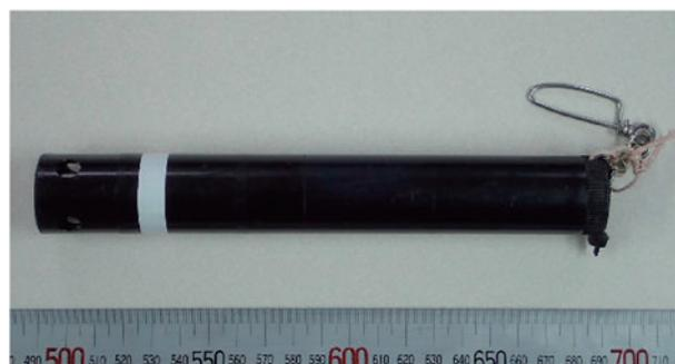
Figure 11. The Temperature Depth Recorder (TDR).
