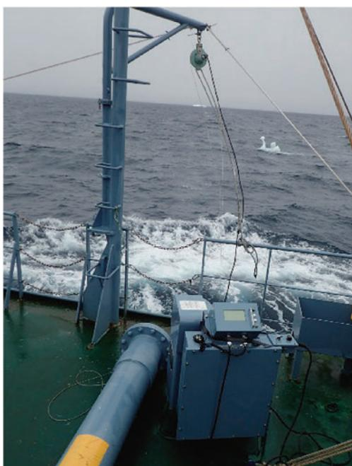
Figure 5. The electrical winch at *Yushin-Maru No. 3*.
