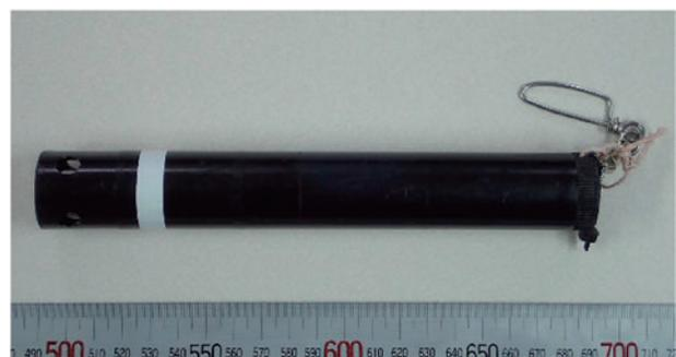
Figure 11. The Temperature Depth Recorder (TDR).
