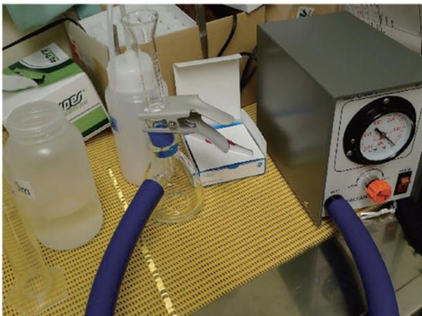
Figure 16. Filtrating seawater with filter paper.
