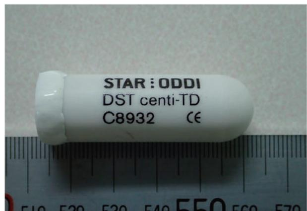
Figure 10. The Data Storage Tag (DST).
