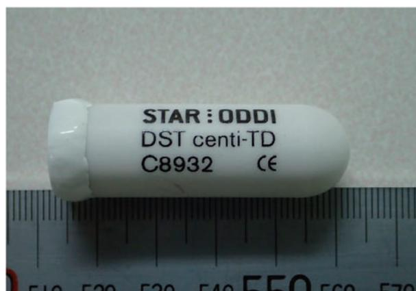
Figure 10. The Data Storage Tag (DST).
