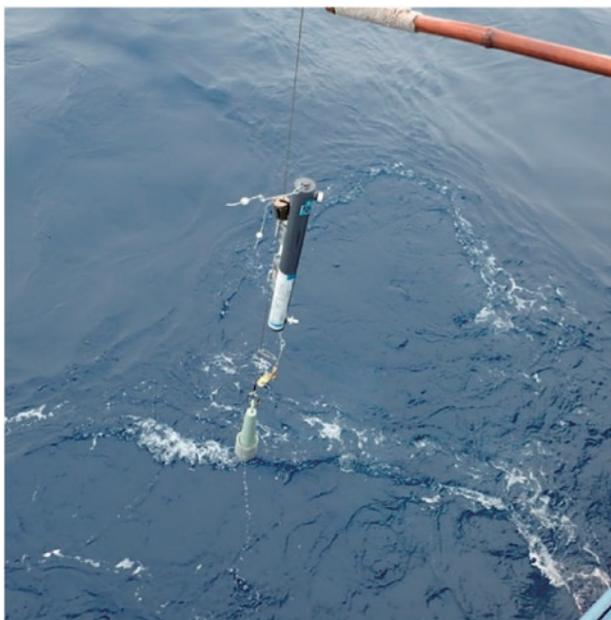
Figure 14. Niskin water sampling bottle at *Yushin-Maru* No. 2.
