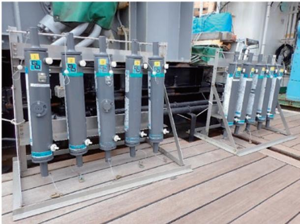
Figure 15. Niskin water sampling bottle at *Kaiyo-Maru* No. 7.
