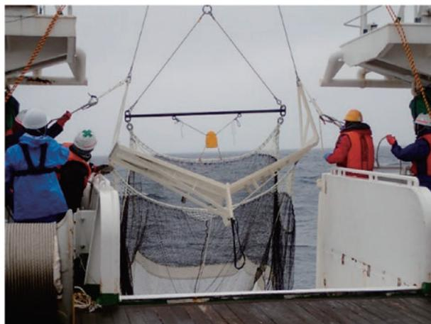
Figure 7. IKMT sampling net at the *Kaiyo-Maru No. 7*.
