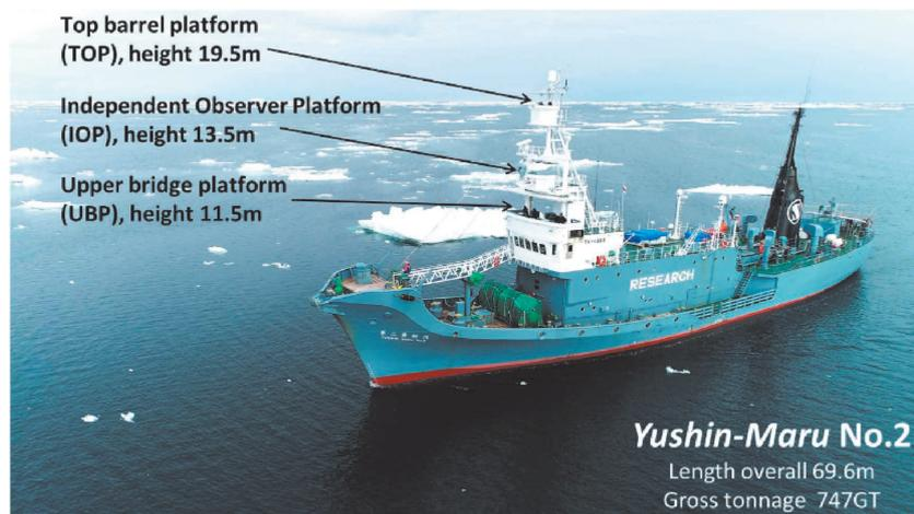
Figure 4. Specifications of the dedicated sighting vessel *Yushin-Maru No. 2*, which is similar to *Yushin-Maru No. 3*.
